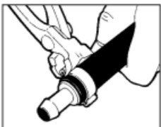
Give each ear a firm squeeze with your Oetiker Standard Jaw Pincers.
