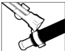
Cut ear by taking several small bites at its base with either pincers. Then grip ear firmly and twist off.
