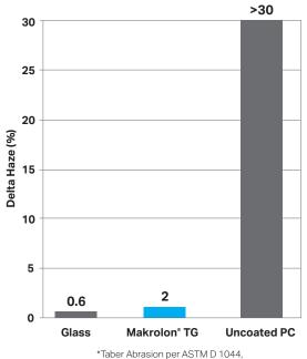
100 cycles using CS-10F wheels at 500 g load
