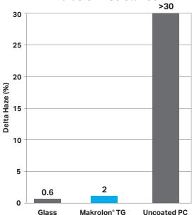
\*Taber Abrasion per ASTM D 1044, 100 cycles using CS-10F wheels at 500 g load
