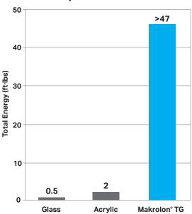
\*Instrumented Impact per ASTM D 3763, sample thickness is 0.125 " nominal
