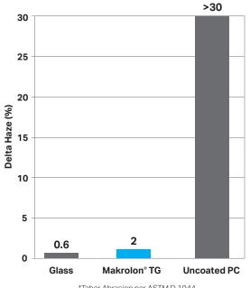
\*Taber Abrasion per ASTM D 1044, 100 cycles using CS-10F wheels at 500 g load
