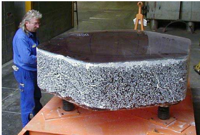
Figure 3: SUPERTEST ZD® near net shape raw casting
