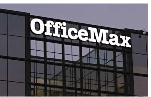
To make the signfaces, the shop used custom-cut sheets of CYRO's ACRYLITE Signflex impact-modified acrylic because of its light-transmission properties. Creating channel letters without hotspots is an important consideration.
