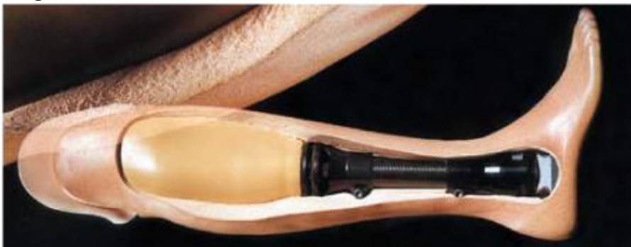
Prosthesis utilizing LD24 Plastazote foam
