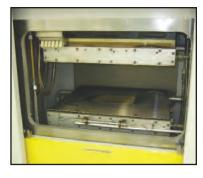
processes. An in-house high temperature vacuum laminating press system allows bonding of the APTIV film to the substrate without the use of adhesives. The versatility to produce multi-layer substrates incorporating APTIV film allows engineers to develop solutions tailored to their specific needs.
