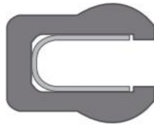
U-Spring type radial and face type seal from 1/16 up to 1/2 inch
