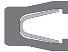
V-Spring type radial and face type seal from 1/16 up to 1/2 inch
