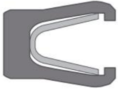
W-Spring type face type seal only from 3/32 up to 1/2 inch
