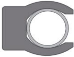
H-Helicoil spring type radial and face type seal from 1/16 up to 1/2 inch
