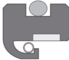
Lipseals sizes according to DIN 3760
