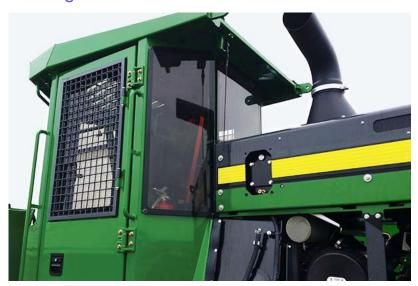
Because of their high impact strength and excellent light transmission, Makrolon® polycarbonate sheet products offer an unsurpassed level of security to any transportation glazing application. To meet the demand for a polycarbonate sheet grade that offers high abrasion resistance and ink adhesion, Covestro has developed Makrolon® Frit Polycarbonate (FP) sheet.
