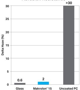
\*Taber Abrasion per ASTM D 1044, 100 cycles, CS-10F wheel
