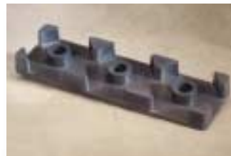
Picture 2 - Most details on this 16" long x 1-1/2" thick spring cap were cast to size.
