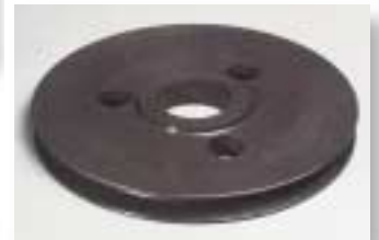
Picture 3 - This 19" diameter Nylatron® GSM sheave requires only finish machining of the bore for bearing press fit.
