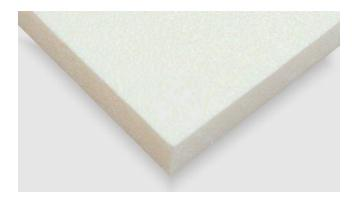
**Foamlite® G** is a **PE-HD-based** lightweight plastic sheet. With a density of 0.75 g/cm³, Foamlite® G has a **weight advantage** of more than 20 per cent compared with compact polyethylene at 0.95 g/cm³. The material boasts a superior **surface quality**, is optionally available with a smooth or grained finish and is **very easy to process**. At the same time, Foamlite® G can be welded with polyethylene (PE) very easily.
