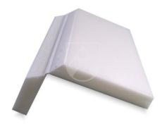
**Integrated Hinge:** Foamlite® P has an "integrated" hinge. It is sufficient to mill a simple 90-degree V-notch into it. The high bending fatigue strength of the material means that the hinge can be folded more than 40,000 times without breaking.
