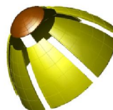
Radome made from honeycomb core details formed
