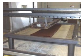
Steel tool for honeycomb heat forming
