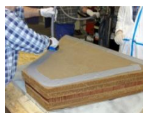
Bonding of honeycomb sheets with paste
