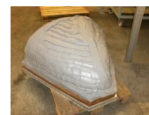
Application of paste on the blank mold
