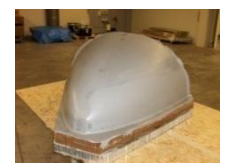
Finished mold after final milling
