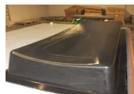
RI-mold for parts made with oven or autoclave curing
