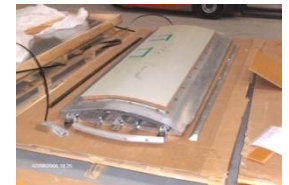
Metal mold for oven or autoclave curing
