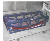
Heat-forming of Honeycombs
