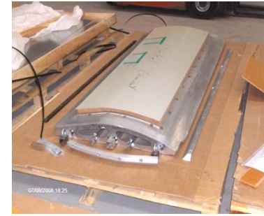
Metal mold for oven or autoclave curing
