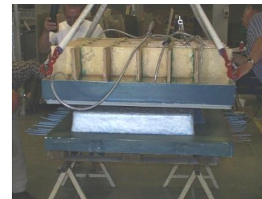
RTM light mold
