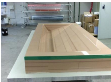
Coated PU tool for model making
