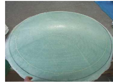
Tool produced with RI for the contouring of formed honeycomb core details
