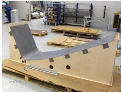
Sandwich part tool for oven curing at 135° C
