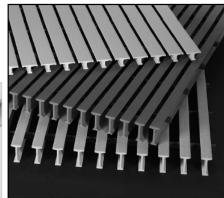
DURADEK® high strength fiberglass grating is a pultruded bar type grating that can be designed and used like traditional metal grates. The individual bearing bars are either 1 or 1-1/2 inch "T" or 2 inch "T" shapes. DURADEK® is a flame retardant product utilizing a premium grade vinyl ester resin. The bearing bars use both longitudinal (glass roving) and multidirectional (glass mat) reinforcements as well as a synthetic surfacing veil to provide unequaled corrosion resistance.
