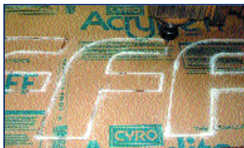
Triangle Sign & Service uses a single-flute Onsrud Cutter bit for fabricating, which gives letters a polished look.
